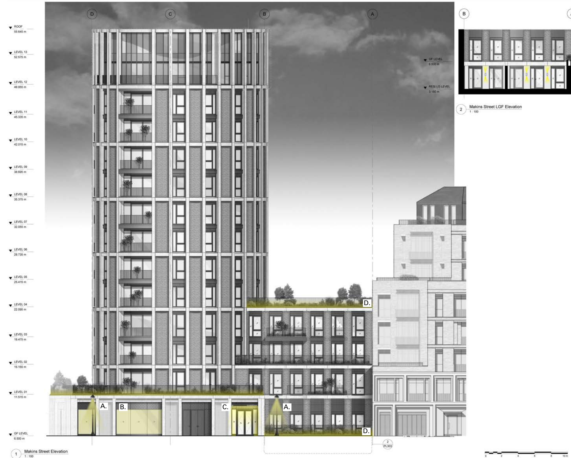
Fig. 7.0.1 - Elevation identifying external lighting elements
